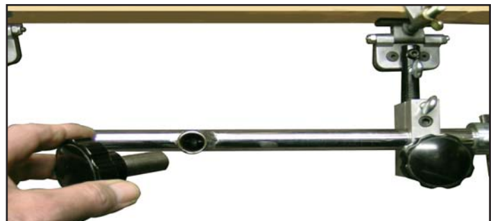
Figure 2. Center knob moves screen frame left to right.
