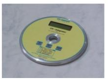
The UV-T Integrator DVD is a self-contained, high quality UV measuring instrument. It is specially designed to measure, record and display peak UV intensity, UV dosage and temperature in the UV curing process of CD and DVD production.
