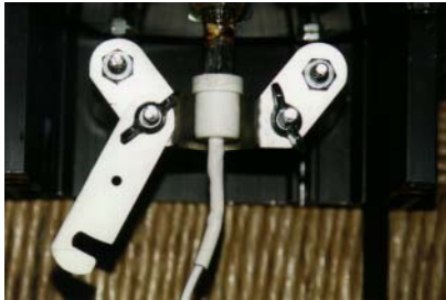
Figure 12: Hold-down bracket unlocked for lamp placement.
