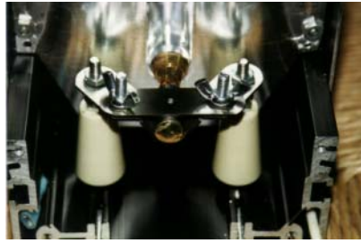
Figure 13: Lamp locked in place; hold-down bracket secured.
