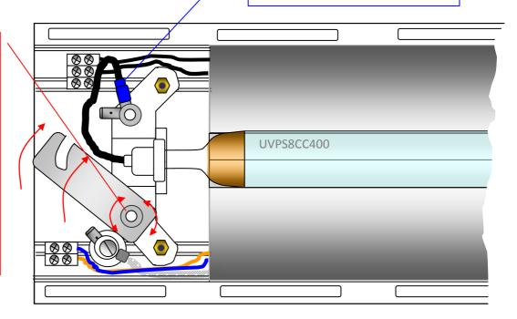
To clamp the lamp in place, swing the top part back into place and gently tighten the thumbscrews.
