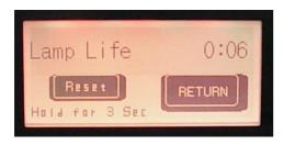
By touching LAMP LIFE on the COUNTER MENU you will go to the LAMP LIFE timer. This should be reset to "0" (zero) whenever you install a new lamp. This timer helps you keep track of the operating hours on your lamp for replacement and maintenance scheduling.
