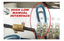
You can activate High or Low from the touch screen during lamp operation (see the "operating your lamp" section) or you can also switch the lamp setting remotely to toggle between High and Low using terminals 23/24
