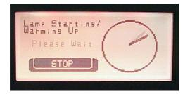
At this point lamp ignition and startup is automated, the lamp starting screen is displayed and the lamp should have ignited and is warming up. (the lamp cooling fan will not be running, this will begin automatically once the lamp is warmed up.
