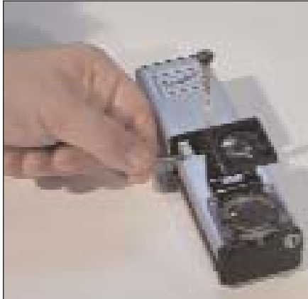
The Pocket Goniometer provides a rapid measurement of static contact angle.
