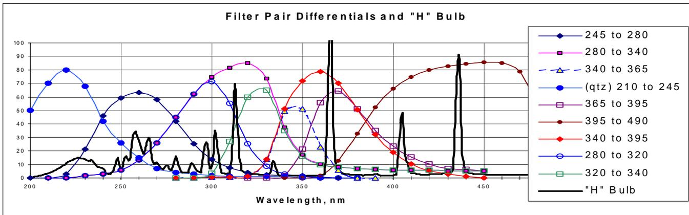
Figure 10. Transmission Differentials of Selected Cutoff Filters and Spectral Output of "H" Bulb.
