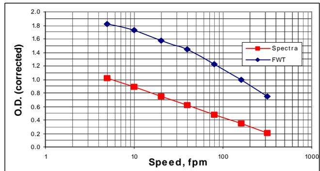
Figure 3. “Linearity” Plotted for SGL Film and FWT Film, “H” Bulb Exposure
