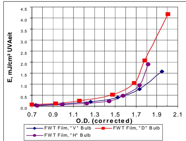
Figure 6. Correlation of FWT Film<sup>(6)</sup> with "H," "D," and "V" Bulbs
