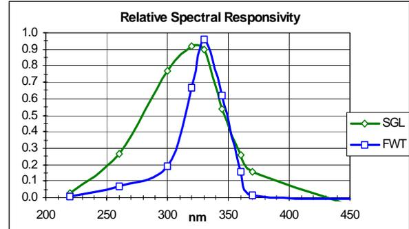
Figure 11. Relative Spectral Responsivity of Two Films
