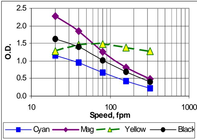
Figure 7. "Quick Check" of Linearity and Dynamic Range, UVTec Film
