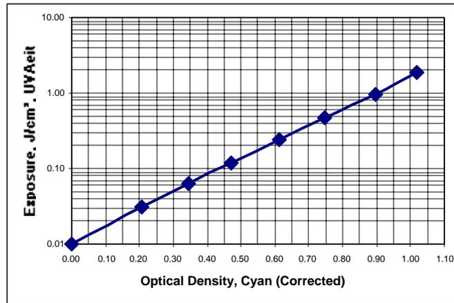
Figure 2 SGL Film<sup>(5)</sup> Exposure vs OD for “H” Bulb
