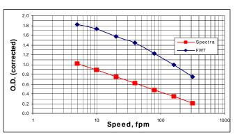
Figure 3. "Linearity" Plotted for SGL Film and FWT Film, "H" Bulb Exposure
