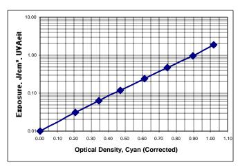
Figure 2 SGL Film<sup>(5)</sup> Exposure vs OD for "H" Bulb
