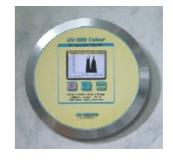
The **UV-1250 Colour ComPort Radiometer + Dosimeter** is a self-contained, high quality UV measuring instrument. It is designed to measure and record UV intensity and UV dosage in the UV curing process. Measuring results are indicated both, graphically and numerically on a big colour display.
