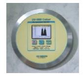
The **UV-1200 Colour Radiometer + Dosimeter** is a self-contained, high quality UV measuring instrument. It is designed to measure and record UV intensity and UV dosage in the UV curing process. Measuring results are indicated both, graphically and numerically on a big colour display.
