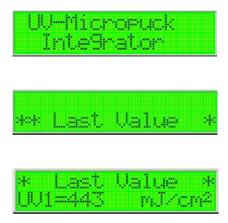
(stored measuring values of the last measuring cycle –example-)
