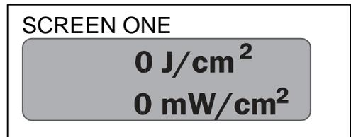
Place the meter **LABEL SIDE DOWN** on the conveyor. When it emerges from the chamber the display will alternate every 5 seconds between numeric and graphical displays similar to screens 2 and 3 to the right.
