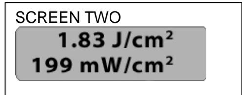
To stop the display from alternating, press “PRESS” **once**. Press it once again to start the display alternating again. The **ILT400/ILT490** will shut itself off automatically after five minutes. To shut it off immediately press “PRESS” **two times** quickly.
