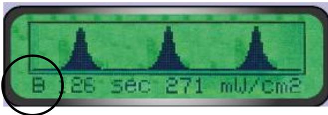
The baseline profile shows all three Lamps having a uniform output of  $271\text{mW}/\text{cm}^2$
