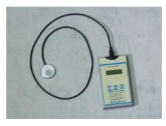
The UV-Microprocessor Integrator TWIN PROBE is a self-contained, high quality UV measuring instrument. It is designed to measure and display the actual UV energy of a UV light source in mW/cm<sup>2</sup>. An additional function is the scan of the peak value of UV-energy in mW/cm<sup>2</sup> and to measure the UV dose in mJ/cm<sup>2</sup> within a pre-set period of 30/60 seconds, or with a triggered scan. (UV-integration)
