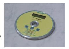
The UV-T ComPort Integrator DVD is a self-contained, high quality UV measuring instrument. It is specially designed to measure, record and display peak UV intensity, UV dosage and temperature in the UV curing process of CD and DVD production.
