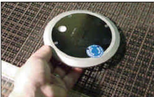
Place DISKURE 365 on conveyor with sensor facing UV light source.
