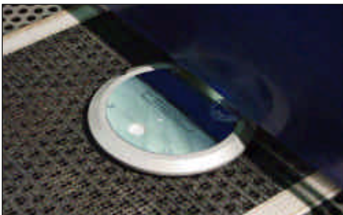
Pass the DISKURE 365 through your curing chamber at same speed your product is being cured to receive an accurate measurement of curing energy.
