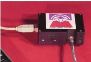
3) The Basic Optical Probes are available as small as 1/4" diameter by 3/4" long, intrude only 3/8" into the curing system, and are easily installed inside the curing zone, anywhere around the lamp. Using a proprietary lens system that interface with the connecting Fiber Optic cabling, Basic Probes will withstand up to 400°C, and come in 4 levels of Optical Attenuation, designed to address very high UV light levels when used in High Energy (300+ watt) lamp systems.
