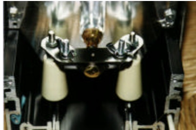
Lamp locked in place; hold-down bracket secured.
