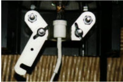
Hold-down bracket unlocked for lamp placement.
