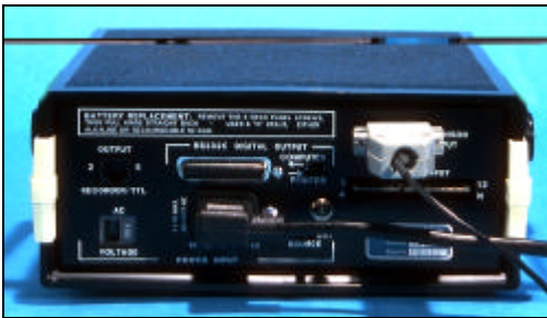
IL1700 Radiometer (back): with Photosensor & Power cables connected
