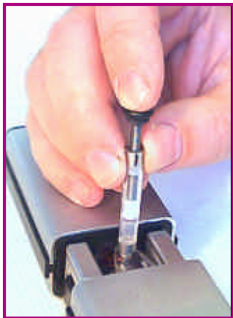
A liquid droplet is projected on a built-in screen for quick analysis.
