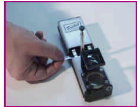
The Pocket Goniometer provides a rapid measurement of static contact angle.
