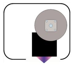
The Rotator is a unique solution for shuttering Lighthouse irradiators in any length. Using a specially designed secondary housing that acts as a light trap, the Rotator prevents unintentional exposure to other areas of the equipment or substrate and effectively protects the operator when production is paused.
