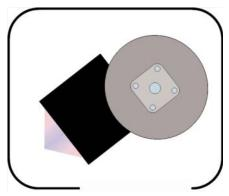
If the operator needs to shut down production for any reason, the inner housing is rotated away from the opening and all UV energy is "trapped" within the outer housing. By pivoting the entire inner housing, we are redirecting the focus of the UV Lamp away from the substrate. Furthermore, in this Standby/Park position, power to the lamp is reduced to the lowest setting, eliminating potential overheating of the irradiator.
