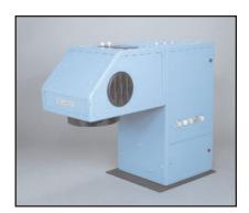
The 1000W Solar Simulator closely reproduces the solar spectrum from 250 to 2400nm using high stability Xenon short arc lamps. It includes a 1000W Xenon lamp and a precision power supply. This benchtop unit provides auto start and adjustable current regulation for variable intensity. An internal electric shutter and an ellipsoidal mirror capture up to 85% of the lamp output. Lamp cabinet access covers are safety interlocked.
